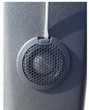
**8** In A-pillar upper region remove the screw and loosen the panel shown.
