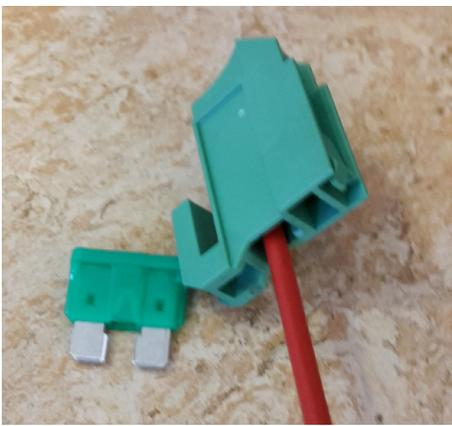
**14** On the reverse side of the Body builder Power Central, insert the fuseholder with cable in an unoccupied position. Make sure it snaps into position. From the front side, insert a 30 A fuse.
