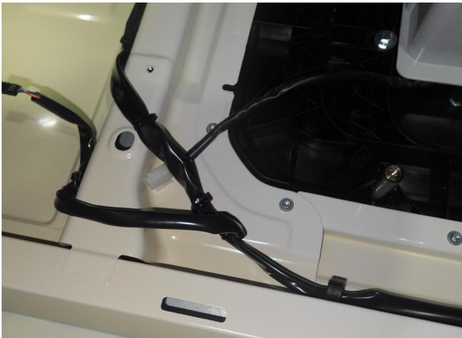
**6** Rout cable along existing cables and structures in the roof area towards the front right part of the cab. Position the cable between the side panel and the storage above the windscreen.
