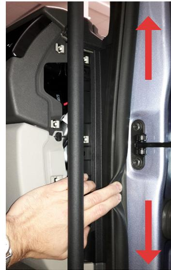
**11** Remove cover to power central, to the right is the Body Builder Power Central, highlighted with a red frame. Remove the two screws and pull out this unit.
