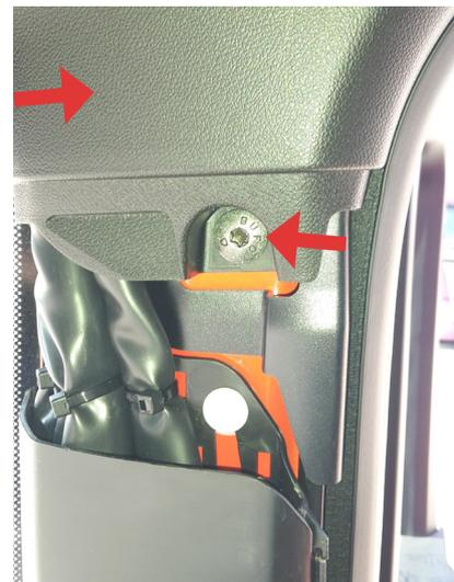
**9** Rout the cable inside the A-pillar cover along with other cables.
