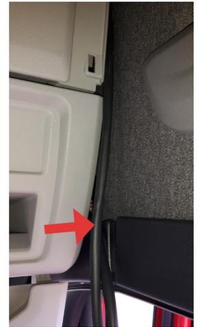
**7** On the A-pillar cover, remove speaker and the screw behind the speaker. Then remove the panel.
